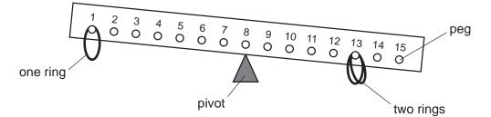
The wooden rod is uniform and all the rings are of equal mass. Two rings are hung on peg 13 and one on peg 1.
